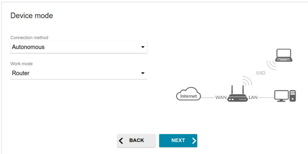
Figure 33. Selecting an operation mode. The **Router** mode.
