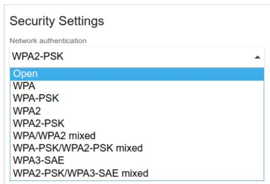
Figure 101. Network authentication types supported by the router.
