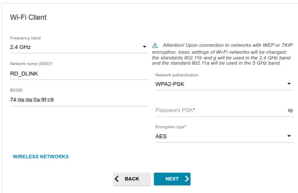
Figure 42. The page for configuring the Wi-Fi client.
