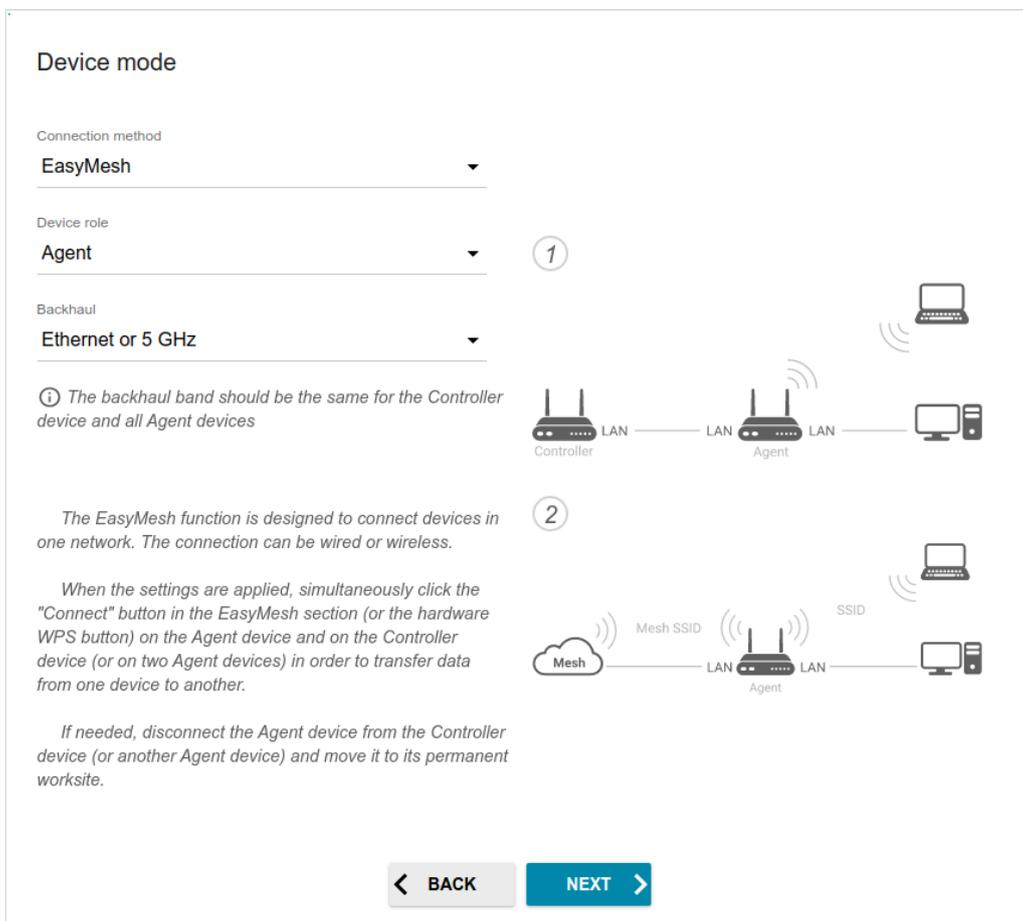
Figure 40. Configuring the EasyMesh function for a subordinate device.
