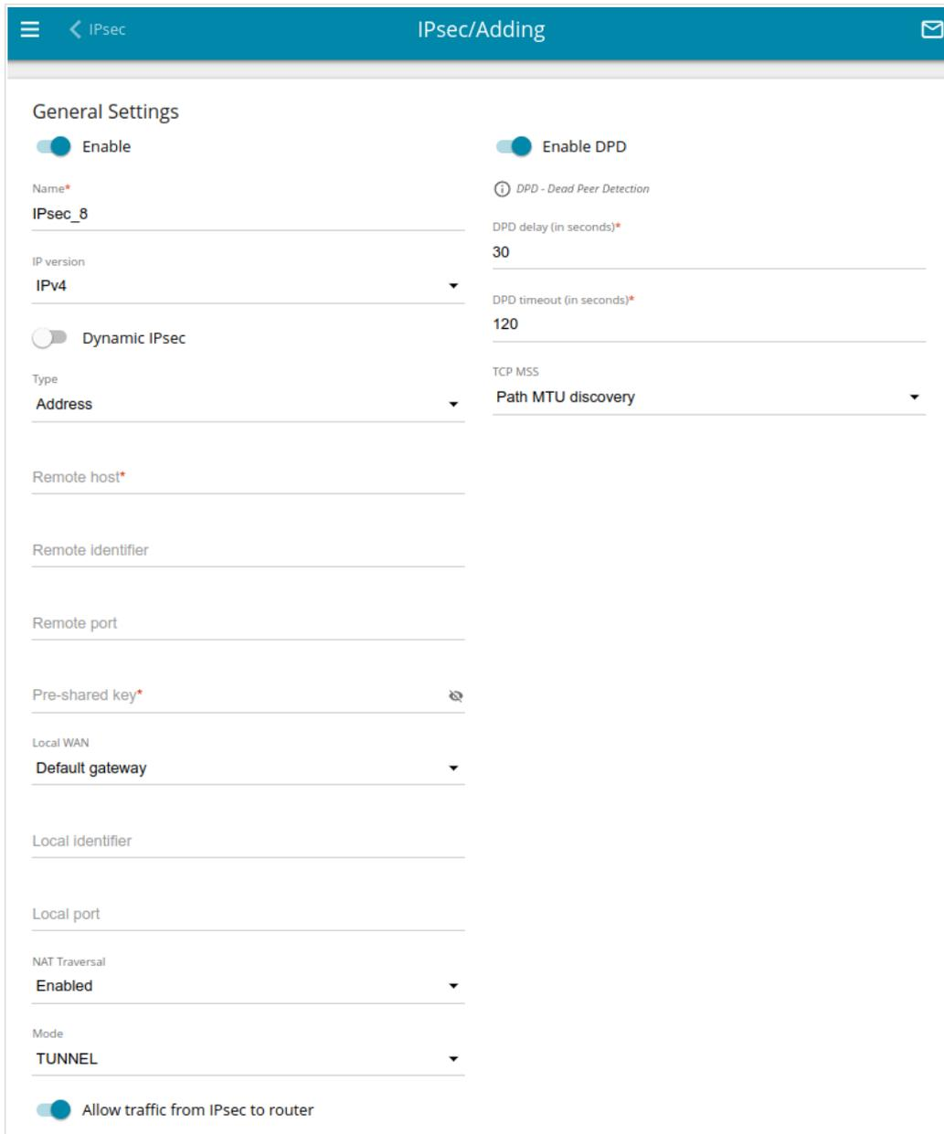
Figure 135. The page for adding an IPsec tunnel. The **General Settings** section.
