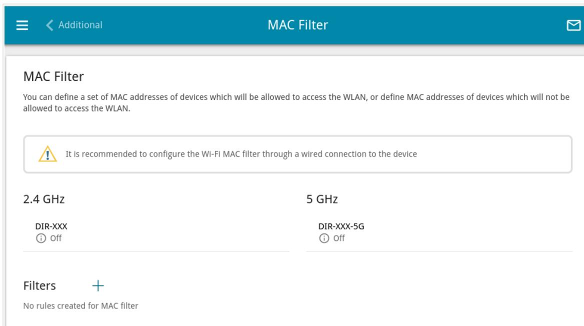
Figure 113. The page for configuring the MAC filter for the wireless network.
