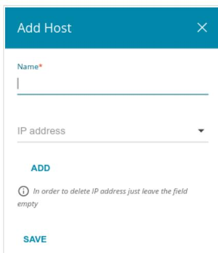
Figure 92. Configuring the local interface. The **IPv4** tab. The window for adding a DNS record.
