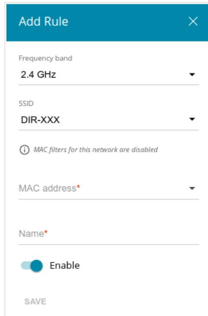
Figure 114. The window for adding a rule for the MAC filter.
