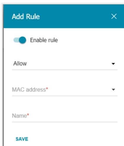
Figure 149. The window for adding a rule for the MAC filter.
