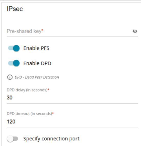
Figure 81. The page for creating a new **L2TP over IPsec** connection. The **IPsec** section.
